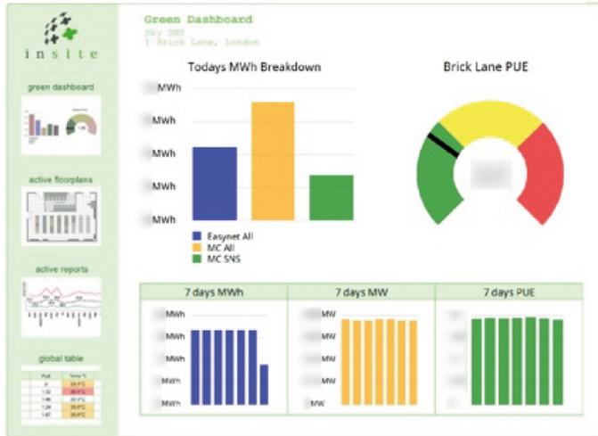
The data centre has 26 PDU panel meters which needed to be monitored 24x7 for parameters such as per phase volts, amps, kVA, kW, kWh and Power Factor. Furthermore, thresholds were to be set which, if breached, would trigger automated alerts via email and SMS text messages. InSite was installed on a server and configured by AdInfa to monitor the PDU meters using SNMP. The primary dashboard is based on an electrical schematic that SNS had and brings it to life by displaying live values.
