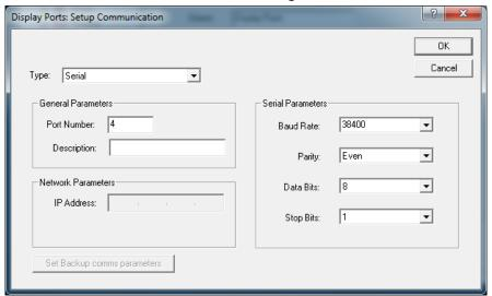
Serial Port 4 addresses all of the RJ45 ports on the rear of the TallyMan.
