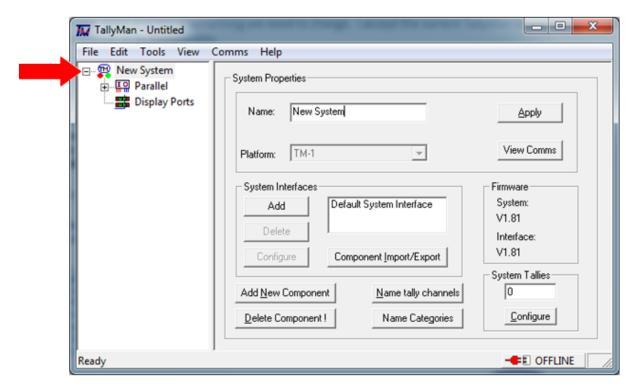
In this configuration a TM1 has been selected so Parallel Tally and Display port components have been generated automatically. The Parallel Tally has been set as 32 in 32 out as default and the display ports set to port 4, port 4 addresses all of the 8 RJ45 display ports on the rear of a TM1.
