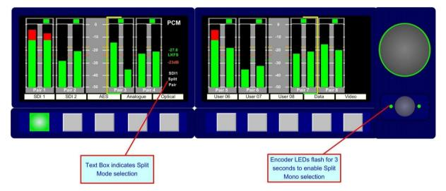
**Note; Split Mono** selection uses the **Assign Matrix** section of the **PAM2-3G16** in order to create a pair of non consequential audio channels. When a **Split Mono** pair is defined, the Assign Matrix represents the resultant signal selection as illustrated below.
