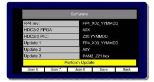
During an update, the left hand **OLED** screen displays the progress of each stage of the installation on a bargraph with a scale 0 to 100%. Front Panel (FP4), FPGA, PIC and Cat552 boards may all be updated via the SD card procedure. Depending on the file size of the update, the procedure may take up to 5 minutes to complete and may appear to have stopped – this is perfectly normal.
