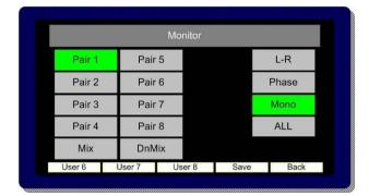
2.6.4 When **Mix Mode** is activated, multiple bargraph pairs may be selected and monitored as a mixed stereo pair.
