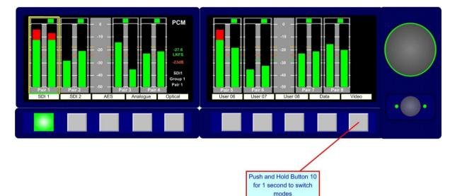
The display changes depending on the whether the signals currently monitored are **Dolby E, D, DD+** or PCM audio. The images below represents the front panel view for Dolby encoded signals and PCM audio respectively.
