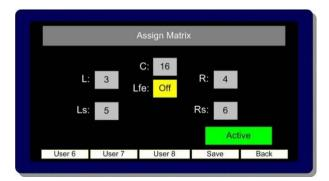
The icons within the **Assign Matrix** screen represent individual channels of a 5.1 programme – by selecting each individually via the encoder, any mono input audio signal can be routed to that output channel. Output channels can be muted if they are not required (as **Lfe** in the example shown).
