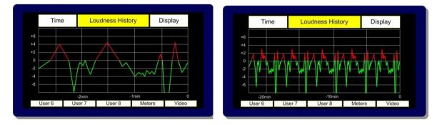
Any measured values which exceed the **Target** level are shown in red. Over **Target** values which then exceed **Limit** are then clipped and do not extend to show peak. This gives the user a comprehensive and instantaneous reference to the behaviour of audio within the tested programme material.
