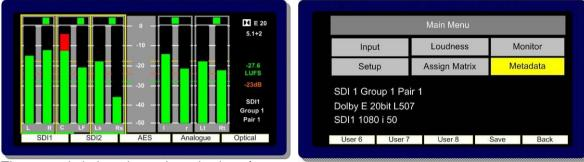
The example below shows the selection of Dolby E PGM 1 as the default for the Metadata screen associated with the selected 5.1 audio signal.
