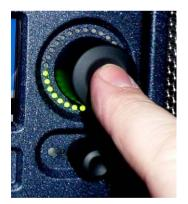
The **Setup 2 Menu** contains a button to select the operational brightness of the switch and encoder LEDs. By selecting and rotating the encoder the overall brightness of the LEDs may be changed from low to high level across 5 graduations. 1 is low, 5 is high.
