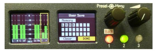
To recall a **User Preset**, rotate the **Encoder** clockwise to activate the **User Preset** window in the right hand OLED screen. Highlight and select to recall a **User Preset**.
