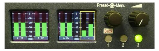
Press the **Encoder** to access **Main Menu.** The encoder is then used to highlight and select from the displayed **Menu** options. From any **Menu**, pressing **Hotkey 1** (illuminated red) will exit the current menu page.
