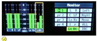
**Dolby** monitoring modes allow the user to select to hear individual audio pairs and stems. The example in the screenshot below shows how to 'solo' the **Centre Channel** and listen to it through the internal or external loudspeakers.
