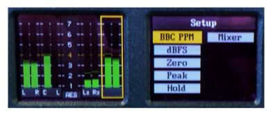
The **dBFS** parameter can be used to alter the 0dB reference level from between -12 and -24 dBFS. The **Zero** parameter selects the offset level between the **Zero dBFS** setting and the onset of **Peak** indication (the point where the bargraph changes colour to red).
