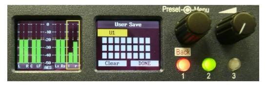
The text boxes in the **User Save** menu can be used to name a **User Preset.** Up to 18 letters or numbers are available. The example below shows a memory being named as **Lt Rt.** Selecting and pressing **Done** saves the memory to the chosen location.
