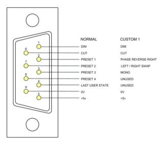
Normal mode is intended to enable instant remote recall of user presets 1-4 from an external manual or automated selector. The ability to remotely **Dim** or **Cut** the internal and external stereo loudspeaker outputs is also featured.
