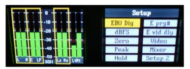
The example below shows the previous **EBU Digital** bargraph scale changed to display a **BBC PPM** bargraph.
