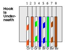
For a hub connection, use a straight-through cable. For TallyMan Controller to Computer, use a crossover cable
