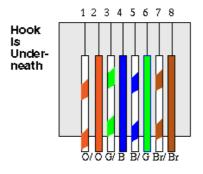
For a hub connection, use a straight-through cable. For TallyMan Controller to Computer, use a crossover cable
