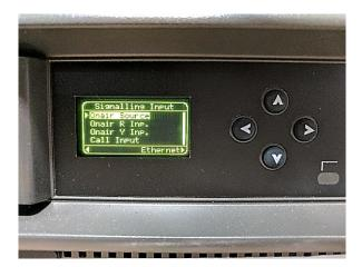
Once 'Onair Source' is selected, use the left and right arrows to choose 'Ethernet' as the on air source signalling input.
