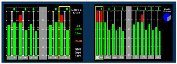
The right-hand display can be altered using the **Shortcut Menu** to show **data**, **video**, **loudness** or **metadata information as required when a Dolby signal is decoded**.
