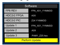
During an update, the left-hand **LCD** screen displays the progress of each stage of the installation on a bargraph with a scale 0 to 100%. Front Panel (FP6), FPGA, PIC and Cat552 boards may all be updated via the SD card procedure. Depending on the file size of the update, the procedure may take up to 5 minutes to complete and may appear to have stopped – this is perfectly normal.
