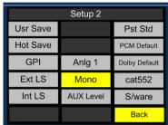
Aux Level: The Aux Level control enables the user to trim the level of the selected Aux Input between 'Off' and +12dB of gain with respect to the signal monitored by the main **PAM1** monitoring function. The level adjustment is graduated in incremental steps as the user pushes and rotates the encoder control.
