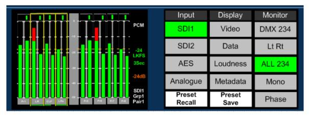
This function ensures that an embedded discrete **5.1** signal can be monitored regardless of the location of the 5.1 stems. The user can store different settings for monitoring discrete 5.1 audio using the **Hotkey** or **User Presets.**
