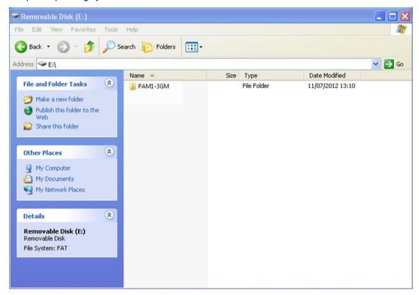
If a storage device is used to upgrade system software within **PAM1** the folder structure will automatically be created in the format shown above.
