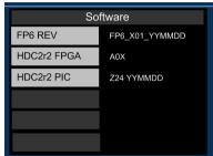
Once the upgrade file is saved, select the **S/Ware** function from the **PAM1 Setup menu 2** and view the current **FP** (front panel) and **FPGA** software versions.
