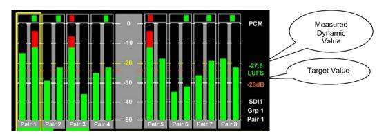
The **Target Level** can be set within a range of +13 to -30 or it can be defined by the **Dialnorm** of a decode **Dolby** signal. The value is displayed as an orange numerical value to the right of the left LCD screen. An orange reference cursor is also displayed across the bargraphs.
