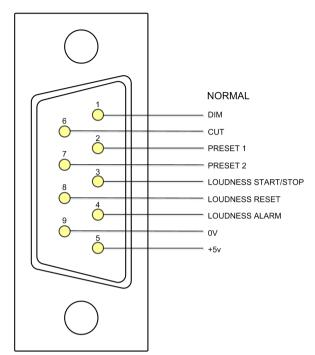
In Momentary Mode, Dim and Cut GPI's latch in a toggle manner, i.e. one closure to ground toggles the function ON: the next ground toggles it OFF. In an ON state: the GPI pin is driven low to allow an LED to be fed from the port. This LED drive is briefly pulsed high at about 100Hz to allow the port to be read whilst it is driving.
