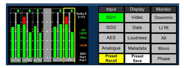
Pressing Preset Recall brings up the 24 User Presets in four pages of 6 presets per page. Each preset is assigned the default user name in the form 'U01: User 01' to 'U24: User 24' however each preset can be allocated a unique user name.
