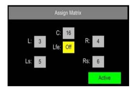
The icons within the **Assign Matrix** screen represent individual channels of a 5.1 programme – by selecting each individually via the encoder, any mono input audio signal can be routed to that output channel. Output channels can be muted if they are not required (as **LFE** in the example shown).
