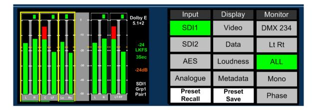
The DRC listening mode can be used in conjunction with either ALL or Lt Rt (Lo Ro) modes and switches Dynamic Range Compression into the monitoring output signal path providing DRC is activated with the Dolby Metadata component of the encoded signal. Line and RF DRC monitoring modes can be selected via the DRC button enabling the user to hear the effect of either form of compression on the decoded signal and hence check the integrity of the audio heard by the consumer.
