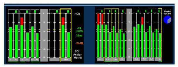
The left hand screen shows a bargraph representation of the output channels with a default condition of a stereo **Downmix** whilst the right hand screen provides a reference to the status of the input channels as defined by the **Assign Matrix**. The sources of the surround sound components are denoted by yellow boxes and text identification below the bargraphs. The setup could then be stored directly to a **User Preset** button for instant recall.
