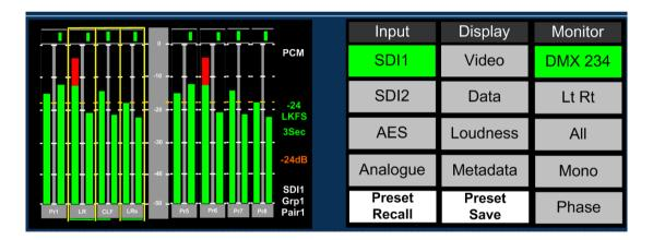
The example above shows how SDI1 pairs 2, 3 and 4 can be Downmixed to stereo
