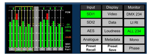
This function ensures that an embedded discrete **5.1** signal can be monitored regardless of the location of the 5.1 stems. The user can store different settings for monitoring discrete 5.1 audio in their **User** and **Hotkey Presets.**
