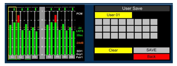
Select the text fields and push / turn the encoder to select alphanumerics or symbols to create the intended name. Once complete simply select **SAVE** and the setup will be saved to the associated memory location
