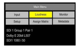
The **Loudness Setup** menu may be used to define the parameters used to measure **Loudness** using the **ITU-R BS1770** algorithm, to select and set the specific audio channels under test and to start/stop measurement manually. The resultant **Loudness** measurement may be observed via either the **Bargraph Display** or from the **Loudness Histogram** which is accessed via the **Data** button.
