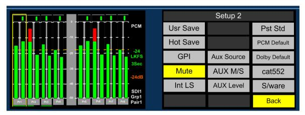
The External loudspeaker (analogue and AES variable level outputs) connections may be muted by using the button located within Setup 2 menu. The action of the on-screen External LS mute switch is preset dependant and not a system default.
