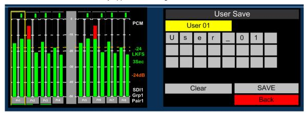
Select the **Clear** button to delete the default or existing text and use the text fields to create a preset or hotkey name to associate with the user setup.
