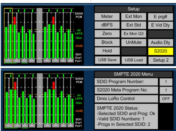
**SDID Program Number:** The SMPTE 2020 status indicator tells the user if any valid SDID are present and also the number (or numbers) from 1 to 9 where 1 is the default and 2 thru 9 represents audio pairs 1 to 8 respectively.
