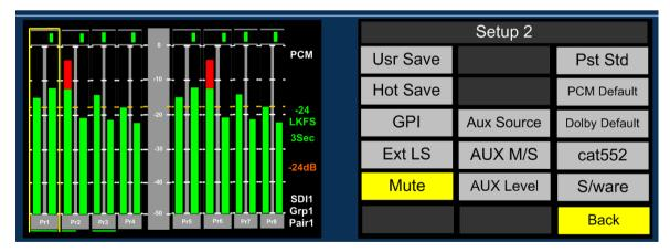
The Internal loudspeakers may be muted via either a rear panel DIP switch or by using the button located within **Setup 2** menu. If the DIP switch is set to 'off' then the function of the onscreen button is defeated. The action of the on-screen Internal LS mute switch is preset dependant and not a system default.
