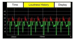
Any measured values which exceed the Target level are shown in red. Over Target values which then exceed Limit are then clipped and do not extend to show peak. This gives the user a comprehensive and instantaneous reference to the behaviour of audio within the tested programme material.
