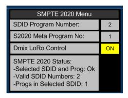
The operator must then activate the PAM downmix feature via the shortcut menu as described elsewhere. With the data page active on PAM1 MK2 the operator will see the following images across the two LED displays.
