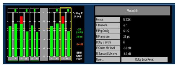
**Scroll to Hear Mode** is used as normal when monitoring **Dolby E, Dolby Digital** or **Dolby Digital Plus** encoded signals. By pushing and turning the encoder the '**Hear Box**' can be moved across the decoded audio channels in the usual way, selecting to listen to **Dolby** components as desired. In the example below, the **Centre** channel has been 'soloed' and would be heard equally from the left and right stereo output channels.
