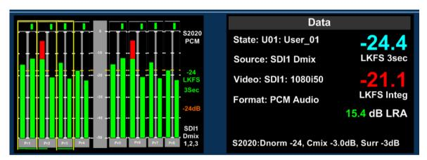
In this example the downmix parameters associated with the S2020 metadata are displayed at the bottom of the data screen alongside the dialnorm value. PAM1 MK2 is using these values to create a stereo LoRo downmix in order for the operator to check the compatibility of the stereo image that will be heard by the viewer at home.
