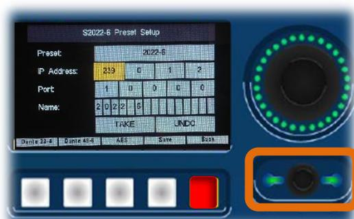
Accessing the Setup Menu on the PAM1-IP-3G is achieved using the pushbutton labelled 'Menu' on its front panel.
