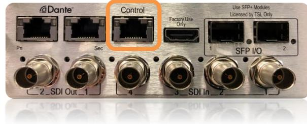
The Control Port can be set to DHCP or a static IP address can be signed using the 'Web Setup' Sub Menu.
