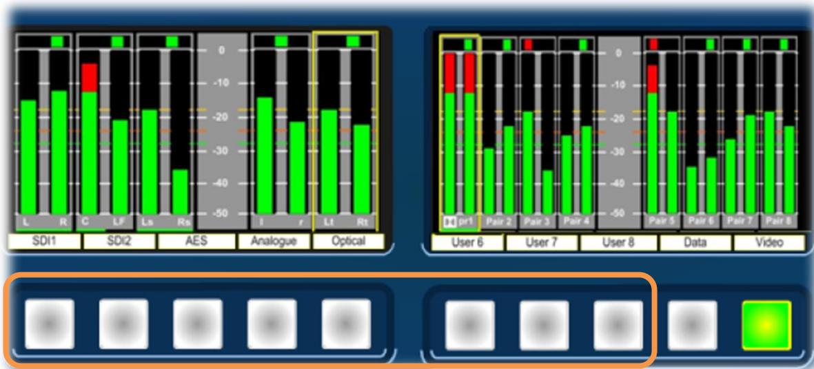
Similarly, up to 24 x SVIP Presets can be recalled using Hot Keys on the front panel of the PAM1-IP-3G. The first 5 SVIP Presets can be assigned to buttons 1-5 on the front panel, with the remaining 19 SVIP Presets accessible using the Preset Recall Menu (accessed using the button labelled 'Shortcut').
