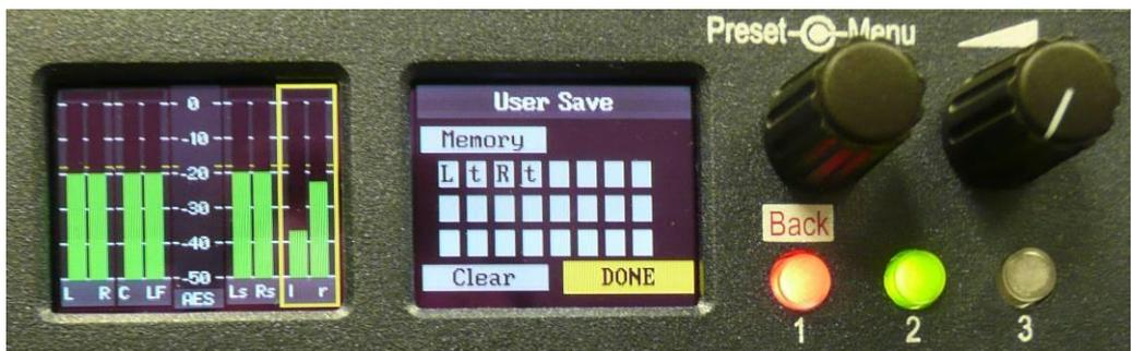
To recall a **User Preset**, rotate the **Encoder** clockwise to activate the **User Preset** window in the right hand OLED screen. Highlight and select to recall a **User Preset**.
