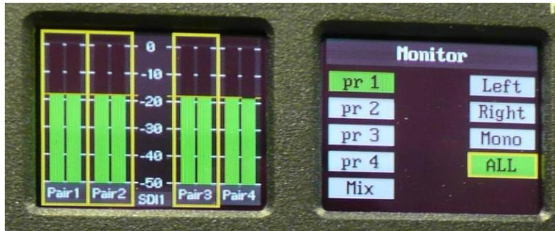
By pressing **ALL** for a second time (illustrated below), the yellow **HEAR** box shifts to highlight an alternative group of 6 audio stems. This function ensures that an embedded discrete **5.1** signal can be monitored regardless of the location of the 5.1 stems. The user can store different settings for monitoring discrete 5.1 audio in their **User Presets**.
