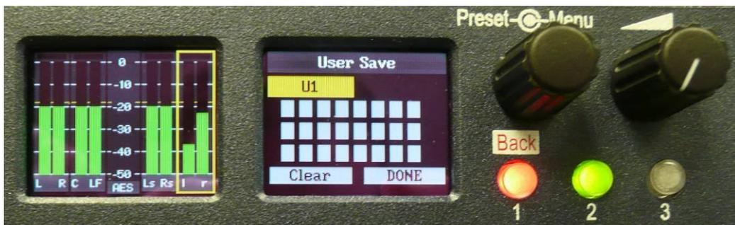
The text boxes in the **User Save** menu can be used to name a **User Preset**. Up to 18 letters or numbers are available. The example below shows a memory being named as **Lt Rt**. Selecting and pressing **Done** saves the memory to the chosen location.
