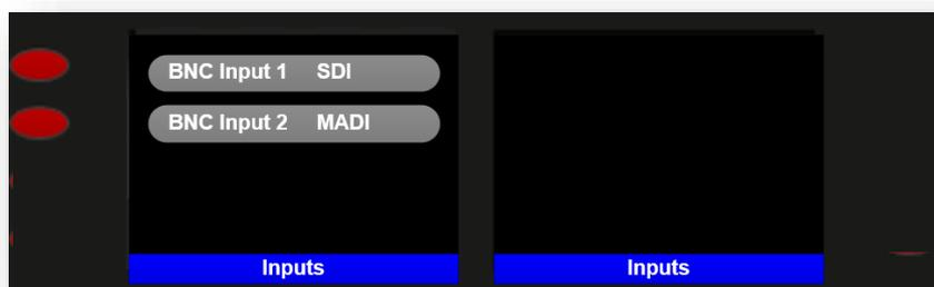
To switch either BNC Input between SDI and MADI, select the Audio Select button for the corresponding BNC Input and rotate the large encoder.
