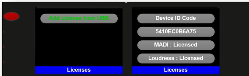
To load a license, simply copy the file supplied by TSL into the root directory of a USB thumb drive, insert it into the front panel of the SAM-Q-SDI and select 'Add License from USB' using Source Select button 1.
