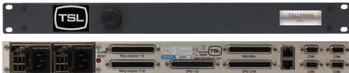
The TallyMan controller should be installed in a standard 19" rack with good ventilation, no other special precautions need be taken, further information regarding earthing, mounting, power etc may be found in the [Safety](#) section.
